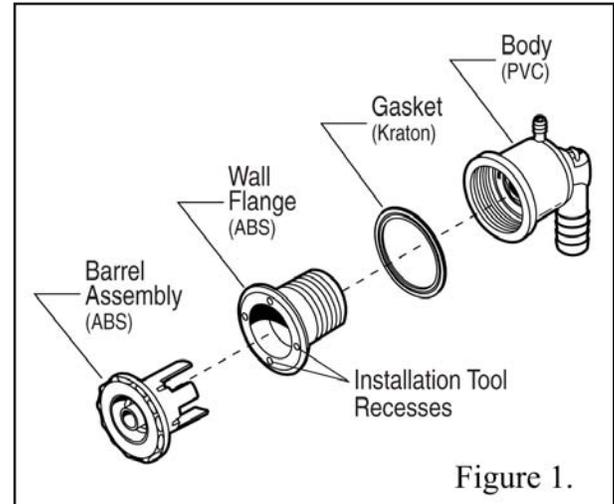
3. Insert the wall flange into the drilled hole. ***It is very important that the spa surface is clean to insure a proper seal between the spa wall and the gasket.***
