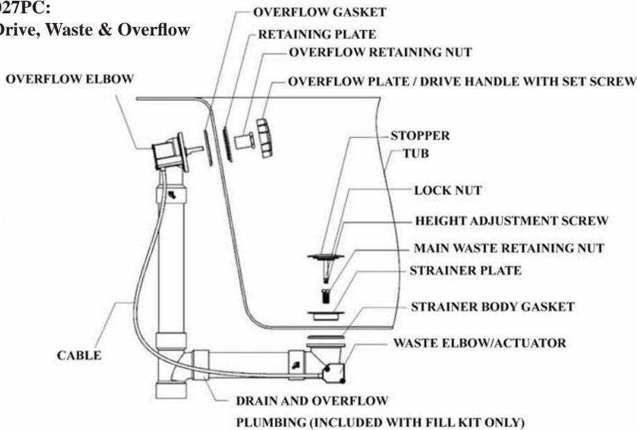
1. INSTALL CABLE ON THE WASHER ELBOW/ACTUATOR AND OVERFLOW ELBOW.
