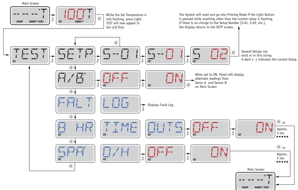
\*If the Control Panel does not have a Warm (Up) button, but rather a single Temp button, use the Temp button in place of the Warm button in the instruction above. (The flow chart assumes a single Temperature Button.)
