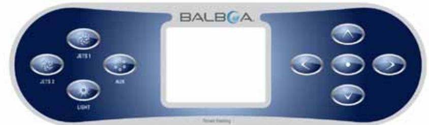
Button labeled "AUX" controls Blower in Setups 2, 4, & 7, and controls Jets 3 in all other Setups.
