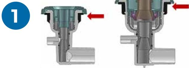
The jet body interlocks with the grommet/gasket to create a slip proof seal, jet will not back out at high temperature and shell movement.
